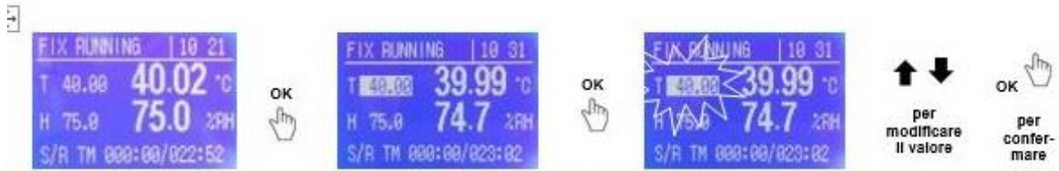
Figure 10 - Changing parameters in FIX mode
