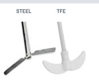
Floating blades The blades open as speed increases, generating downward axial flow. Use: narrow-necked containers, like flasks.
